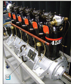
The red bands 11 & 19 are not always clearly visible in archive photos but should be applied around every cylinder to indicate that they are over compressed.
