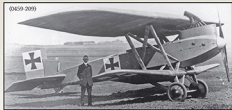
200hp Benz Bz.IV powered Junkers J 4 prototype photographed on 3 May 1917. The J 4 went into production as the armour plated ground attack Junkers J.1 with 227 built by Junkers-Fokker (Jfa) before production was halted in 1919.
