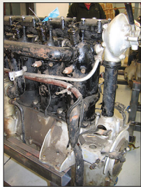
Rear port view showing the empty magneto mounts, water pipe and spark plug details.
