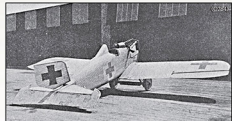
160hp Daimler-Mercedes D.III powered Junkers J 7 photographed on 3 May 1917, now with a nose radiator, new exhaust and post April 1918 balkenkreuz markings. Not visible in this print, the wheel covers of Junkers & Co built J 7 were now curiously marked with "Jfa", most likely representing Junkers-Fokker for political and/or marketing reasons.
