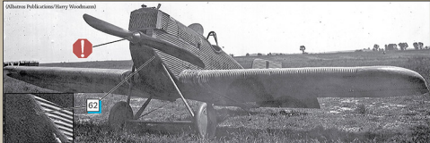
A sole Junkers D.1 was fitted with a 185ps (230hp) BMWIIIa engine in early October 1918 and this photo is thought to show it undergoing flight testing before being entered in the 3rd fighter competition later that month where it performed very well. Note the overall monotone finish (white paint has yet to be applied), lack of armament, Rupp quick release propeller boss commonly associated with the BMWIIIa engine and Heine propeller.
