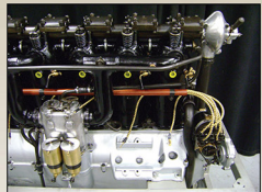
Water jacketed intake manifold and carburetor intake detail. A mount for the generator (94) can be seen at right but the actual generator was very rarely installed in fighter aircraft unless used to power an electrically heated flight suit or wireless transmitter.
