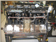
Port side of the engine, the red-brown pipe carries the plug leads from the magnetos to the spark plugs.
