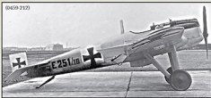
120hp Daimler-Mercedes D.II powered steel skinned Junkers J 2 E251/16 photographed in July 1916. Although six J 2 were built it proved to be too heavy and underpowered for front line use, despite being trialled with a 160hp Daimler-Mercedes D.III engine.
